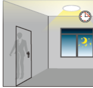
After the desired hold time and there is no new motion detected, the sensor will dim the fixture to a lower light level.
