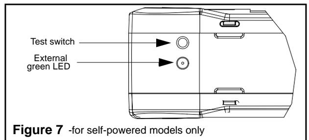
**Figure 7** -for self-powered models only
