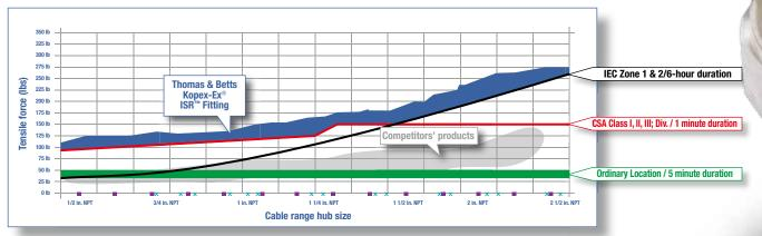
Tensile force vs. cable range hub size
