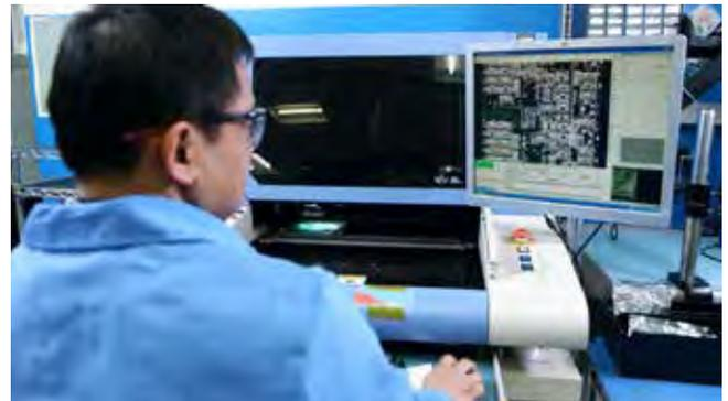
The AOI (automated optical inspection) machine added to our printed circuit board operation is one of the first of its kind in use in North America.
