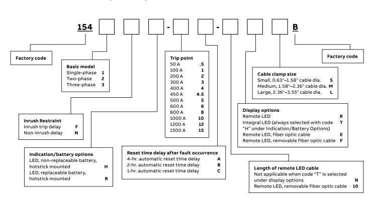
Fisher Pierce TPM series test point fault indicators
