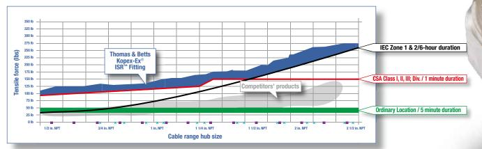
Tensile force vs. cable range hub size
